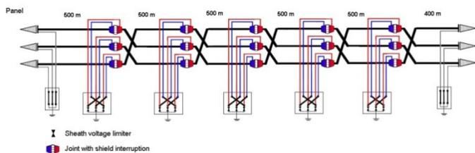
Figure 7 – Scenario I connections scheme (cross bonding)
