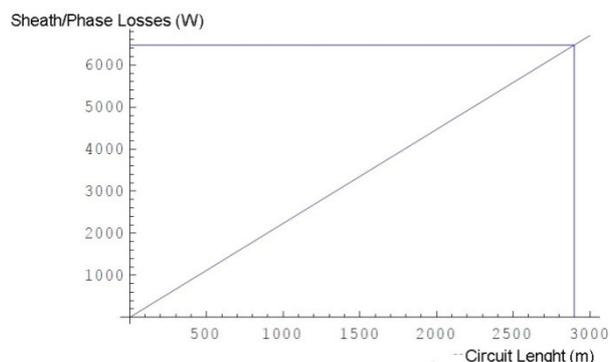
Figure 9 – Shield losses with cross bonding [2]
