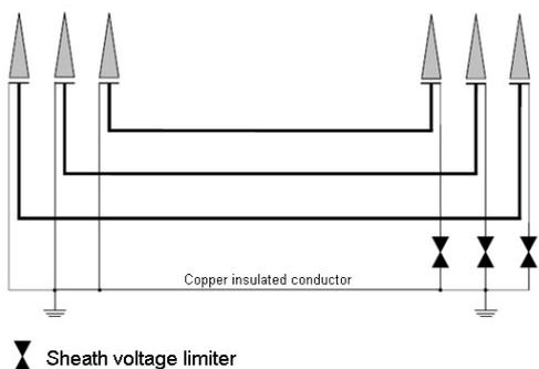
Figure 3 – Single point bonding [2]
