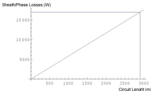
Figure 8 – Shield losses with both ends bonding [2]
