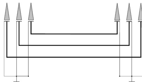
Figure 2 – Both ends bonding
