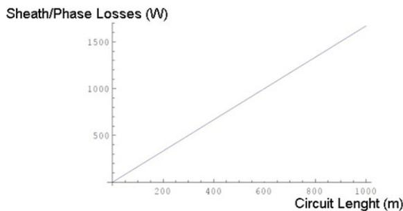
Figure 11 – Shield losses with single point bonding [2]
