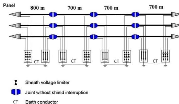
Figure 10 – Scenario II connections scheme (single point)
