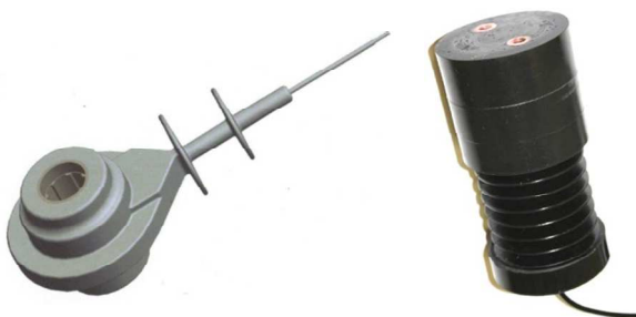
Figure 7: two different prototypes of integrated voltage and current sensors
