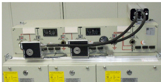
Fig. 3: Adaptive actuator system on switchgear GA F&G (Ormazabal)
