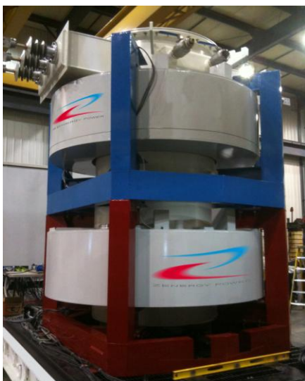
Figure 5. Compact FCL with “dry-cooled” HTS magnets surrounding an oil-filled dielectric tank with AC coils.
