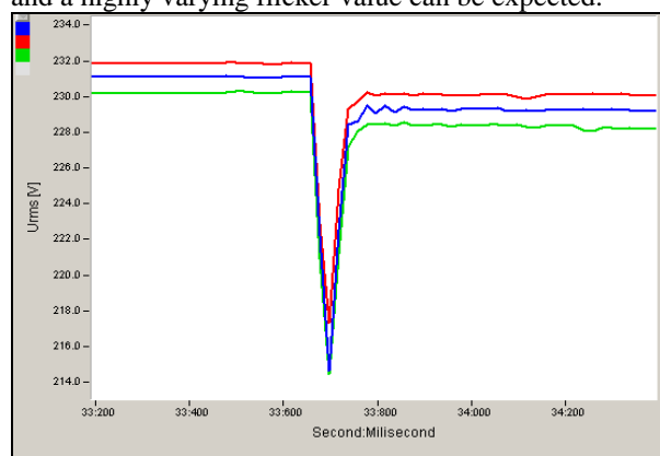
Fig. 5: detail of Urms changes at the time of actuation of an actual heat pump, change duration 100ms, change depth 16V
