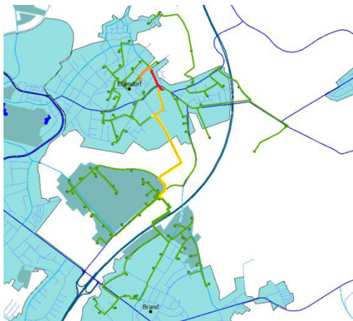
Figure 6: Localised overloads of power grids
