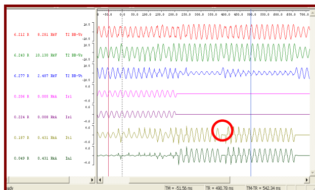
Fig.1: The recorded voltage and current channels – CB Restrike –
