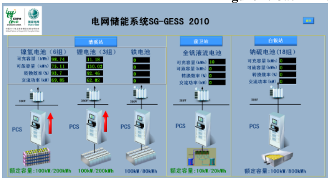
Figure 2. Grid energy storage system (SG-GESS system diagram)
