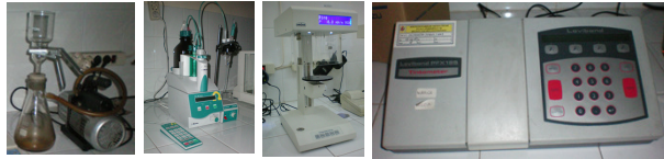
Fig 3. Several test equipment to indicate Transformer oil quality (Sediment, acidity, IFT & Colour)
