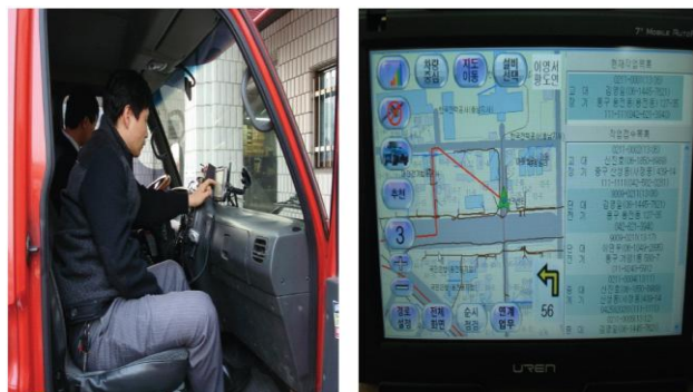
Fig. 4 Patrol Mobile System [displaying the outage point and route using GPS via wire-less communication network]
