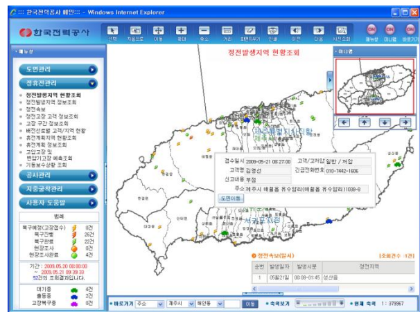
Fig. 3 Outage Monitoring Screen [displaying the position of outage in different color depending on the state of outage]
