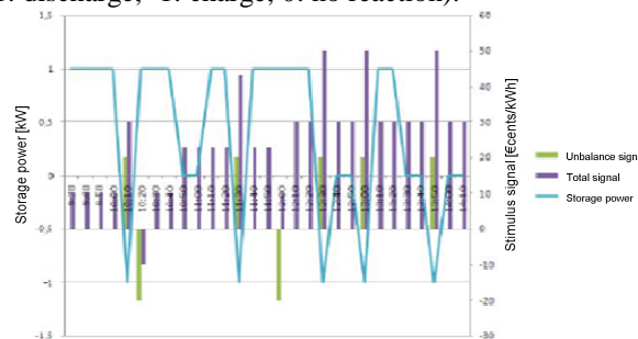
Figure 3. Response of a storage unit on a price based stimulus signal (Low price: charge; high price: discharge; medium price: no reaction)
