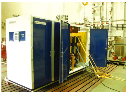
Fig.10 Test of short circuit current
