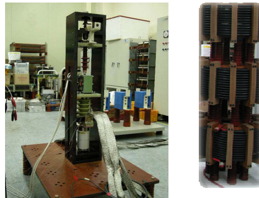
Fig.7 Fast switch module and reactor
