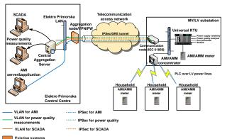
Figure 1: The concept of the integrated MV/LV substation integration through unified telecommunication network
