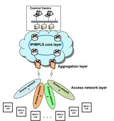
Figure 2: The three level hierarchy of the Elektro Primorska communication network
