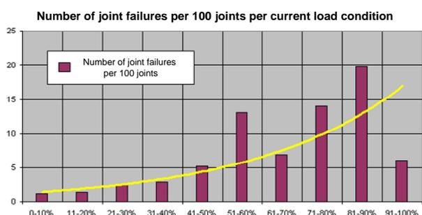
Figure 1 The number of failing joints in relation to the cable load.
