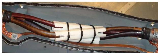
Figure 10 Conductor extension when the force is about 6 kN. The potential degradation of the paper insulation is very likely in case of a cyclic load.
