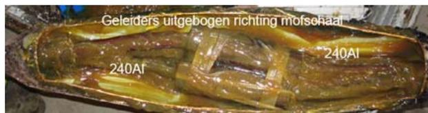
Figure 11 Field result: a similar joint as shown in Figure 10, but failed in service due to conductor extension.
