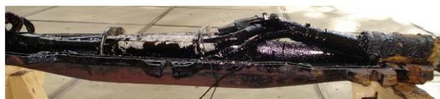
Figure 4 Joint of the type with a bitumen insulation, where the conductor extension was such that the insulation got damaged in the bend of the cores and the joint failed.
