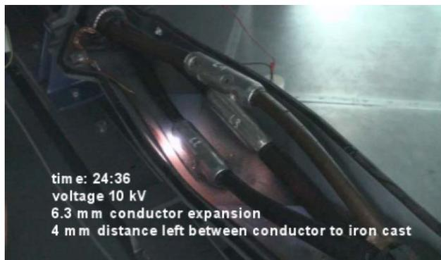
Figure 8 Laboratory result: a conductor extension of 6.3 mm causes a failure in a 10 kV joint (insulation material replaced by air, no upper iron case).
