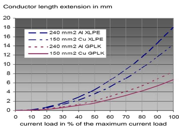
Figure 6 Calculated conductor length extensions as a function of the current load situation for PILC and XLPE insulated cables with a conductor cross-section of  $150 \text{ mm}^2$  or  $240 \text{ mm}^2$ .
