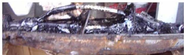
Figure 9 Field result: a similar joint as shown in Figure 8, but failed in service due to conductor extension.
