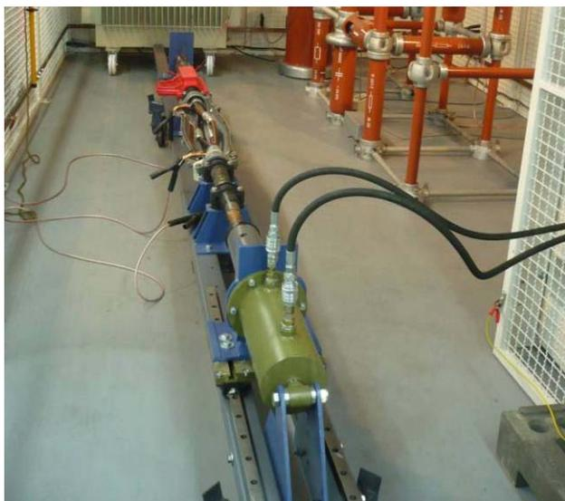
Figure 7 Test set-up where the mechanical forces applied to the conductor can be created by oil pressure.
