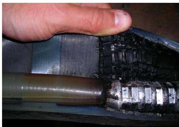
Figure 3 Conductor connector that came loose and thus started to heat its surrounding joint material.
