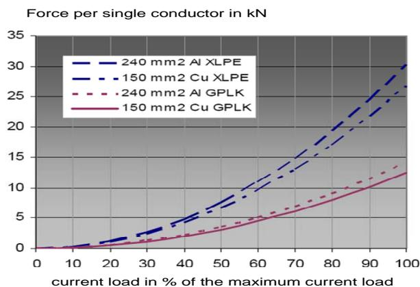
Figure 5 Calculated forces per single conductor in kN as a function of the current load situation for PILC and XLPE insulated cables with a conductor cross-section of  $150 \text{ mm}^2$  or  $240 \text{ mm}^2$ .
