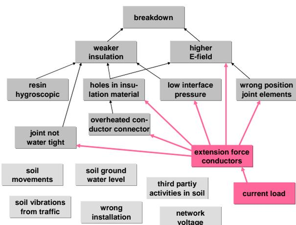
Figure 2 Degradation mechanisms, the high current load is found to be dominant.
