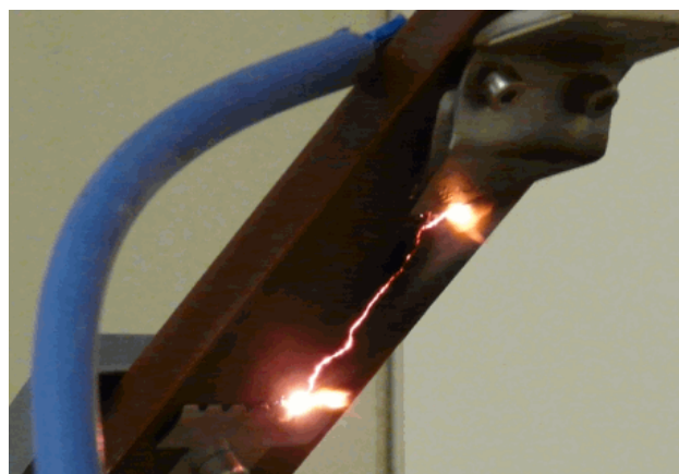
Figure 3: tracking test according to IEC60587 for class 1A2,5 (at 2.5 kV) on polyurethane resin use for SF6 carters and MV instrument transformers.
