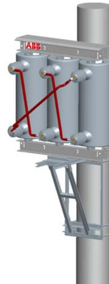
Figure 5. 3D-drawing of a pole mounted transformer installation (from HV side) on a standard \phi = 360\text{mm} single pole.
