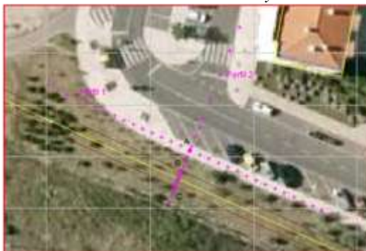
Figure 3: locations of the measurement points (in rose) of the 60kV line in Fig. 2, defined according to [6], where the 3-points were considered as in IEC 62110 [5].
