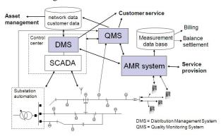
Fig. 1. Using AMR system in network management [2]
