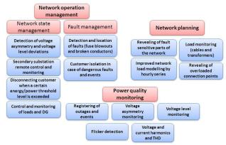
Fig. 2. Utilizing AMI in LV network management.
