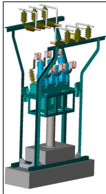
Figure3: Integrated Switching Devices (ISD) in service
