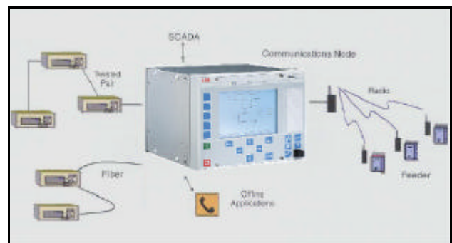
Figure 6: Integration of substation and feeder equipment communications.
