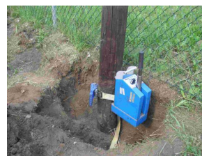
Figure 2: Measurements at ground line level and at -30cm under the ground line level (after digging).
