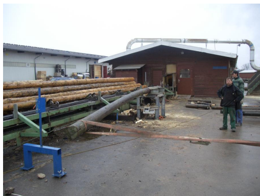
Figure 4: Destructive tests and comparison with Polux residual strength evaluation. Tests in Hüfingen, Germany, Fürstenberg Holz.
