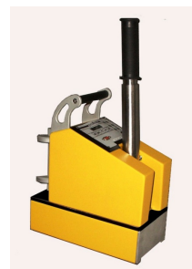
Figure 1: Polux device, 4 th generation. Non-destructive technology for wood pole quality assessment.
