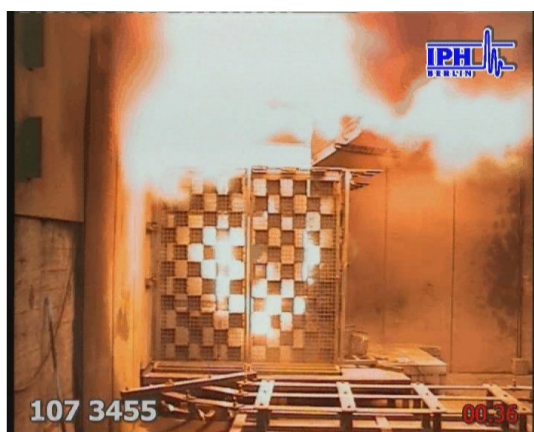
Figure 10: Test with pressure relief into the room without absorber
