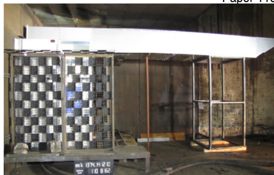
Figure 6: PIX-Panels with exhaust duct
