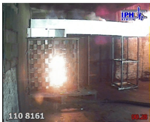
Figure 8: Test performed with 40 kA / 1s in CC, duct configuration
