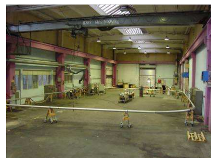
Figure 7 45 m long cryostat with cable model during hydraulic testing
