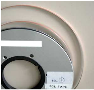
Figure 1 A sample of HTS tape with FCL properties
