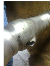
Figure 2: internal gas-pressured cable junction box
