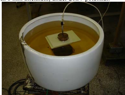
Fig. 1 - Test vessel with polyester slab containing artificial void, placed between two ASTM type brass electrodes and immersed in insulating oil.
