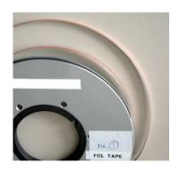
HTS tape conductor can carry 300 A/mm2 at 77 Kelvin
