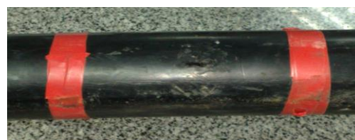
Figure (4) Breakdown during withstand voltage for 66 kV cable after 00:31:55 with 27.05 Hz
