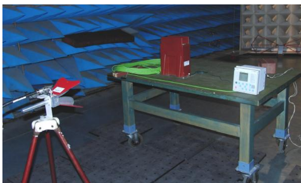
Fig. 7 Electromagnetic field immunity test
