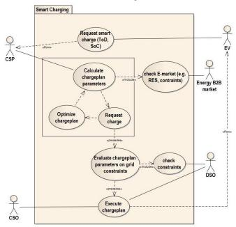
Fig 3: Smart Charging UML use case diagram
