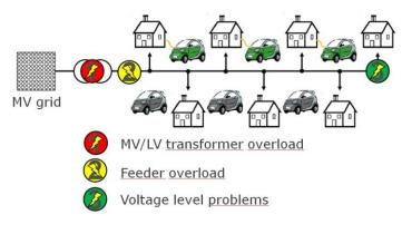
Fig 1: Technical problems related to (large scale) uncontrolled EV charging [3]
