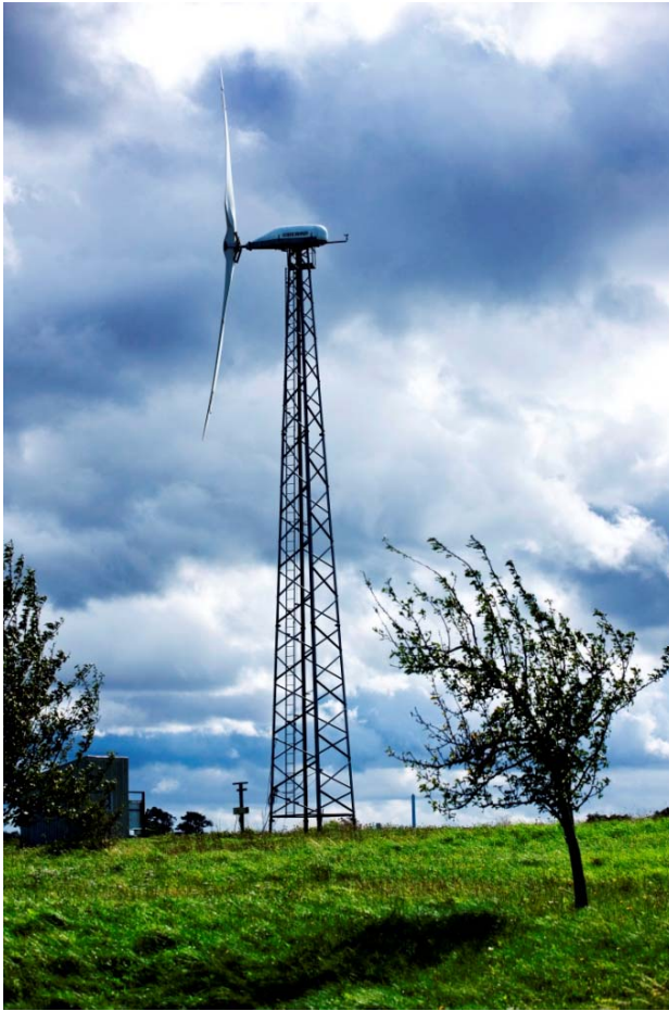
Figure 2: The 11 kW Gaia wind turbine used in the experiment.
