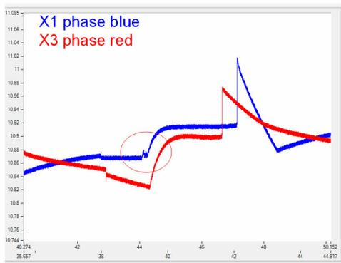
**Figure 8.** DRM trace indicating coking on transfer switch
