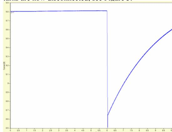
Figure 3. DRM of a tap change from position 4 to 3
