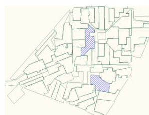
Blocks with critical power losses, and strong dependence between power losses and LV feeder length
