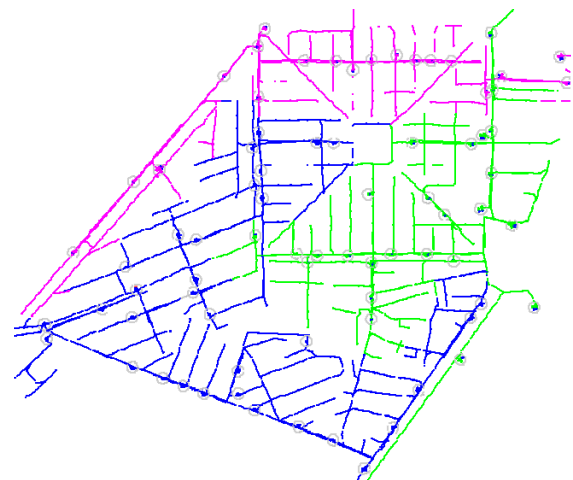
Fig 1: Lashkar Abad distribution network, there are three 11KV feeder that shown with different color, there are also 69 transformer that depicted with circle around them
