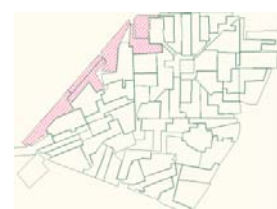
Blocks with critical voltage drop, and strong dependence between voltage drop and LV feeder length
