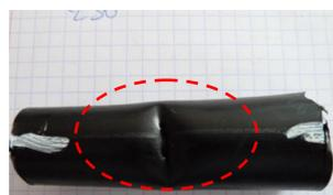
Fig. 13 : LLDPE sheath after impact test (Outer side)
