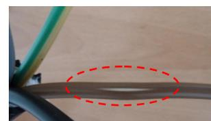
Fig. 14 : Insulation under the LLDPE sheath (after impact)
