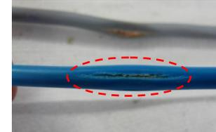
Fig. 16 : Insulation under the PVC sheath (after impact)
