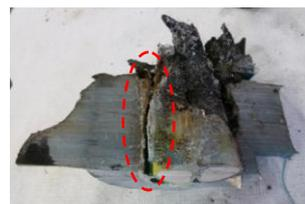
**Fig. 2 :** Poor adhesion between the resin and the XLPE insulation
