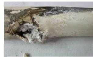
**Fig. 6 :** Degradation due to water ingress
