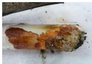
**Fig. 3 :** Corrosion on the PVC filler
