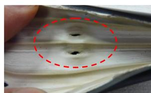
Fig. 15 : PVC sheath after impact test (Inner side)
