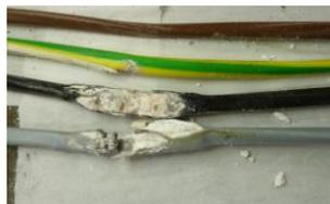
**Fig. 5 :** Corrosion of conductors
