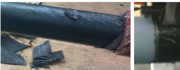
Fig 1. Indentation in/ irregularities on the insulation screen.
