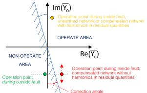
Fig. 1 Operation characteristics of multi-frequency neutral admittance protection, which is valid both in compensated and unearthed networks.
