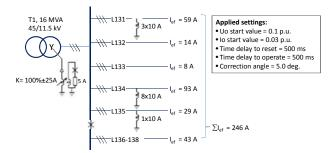
Fig. 4 Parameters of the studied network and settings of multi-frequency neutral admittance protection.
