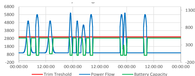
Figure 2: Example profile for ESS testing
