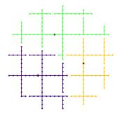
At this point, it is possible to calculate a load flow, but the result has little chance to be realistic, as losses and voltage drop are far beyond acceptable value. **Thicker cables have to be used.**
