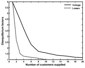
Thus, the load flow used in this paper makes an **equilibrate load flow** using backward forward method, and then voltage drop and losses on each cable **are multiplied by a factor** (one for voltage drop and one for losses), depending on the number of customer supplied by the cable. Disequilibrium factors are parameters of the calculation.
