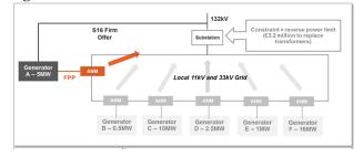
By applying the Reinforcement Guarantee approach, generators can connect in a constrained zone of the network without triggering the reinforcement and instead accepting a level of curtailment of their output. Then, if
