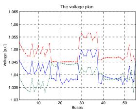
Fig. 2. Initial and final voltage profiles
