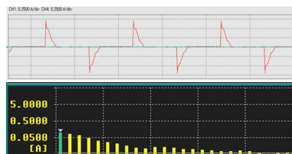
Figure (6) - The current waveform and harmonic spectra for a CFL
