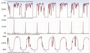
Figure 11 Top; 3.8 kHz component, middle; 4.85 kHz component, bottom; active power. Figure shows one phase during one week.
