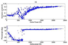
Figure 5 150 Hz component, amplitude and phase
