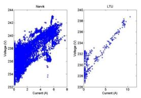
Figure 2 Voltage rise due to increased production
