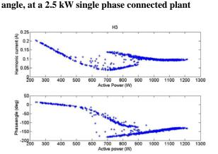
Figure 6 150 Hz component, amplitude and phase angle, at a 1.5 kW single phase connected plant
