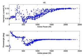
Figure 9 Harmonic five, amplitude and phase angle, at a 2.5 kW single phase connected plant
