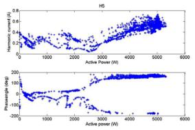
Figure 7 Harmonic five, amplitude and phase angle, at a 20 kW three phase connected plant
