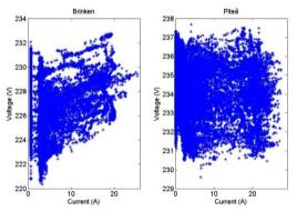
Figure 1 Voltage variation at the two 20 kW three phase connected plants, on the right the fixed system and on the left the system with 2-axis tracking
