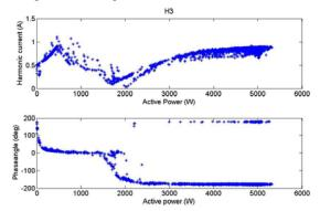
Figure 4 150 Hz component, amplitude and phase angle, at a 20 kW three phase connected plant
