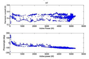
Figure 10 Harmonic seven, amplitude and phase angle, at a 20 kW three phase connected plant
