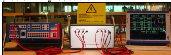
Figure 3 - Test setup with CMC and DEWE
