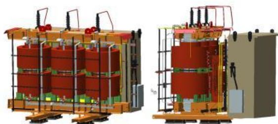
Fig. 9: Views of the 16MVA transformer inside the enclosure
