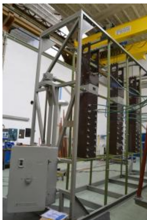
Fig. 2: Dry-type on-load tap changer for the 72.5 kV voltage level, consisting of a switching unit for each phase and a common drive
