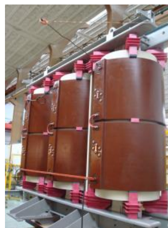
Fig. 1: Dry-type subtransmission transformer: 66 kV / 10 MVA
