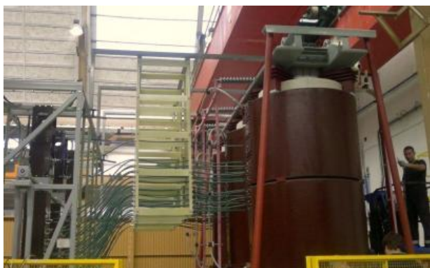
Fig. 8: Final assembly of 25 MVA HiDry 72 transformer and OLTC
