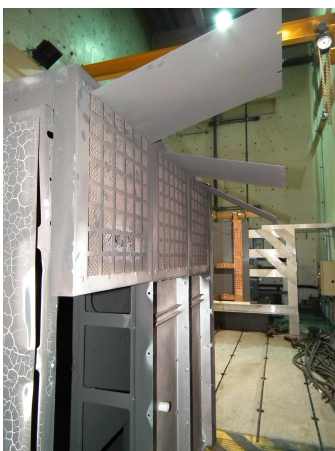
Figure 10: example of a porous type absorber, Schneider Premset range, after internal arc test.
