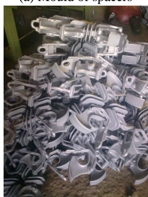
(c) Mass production of spacer
