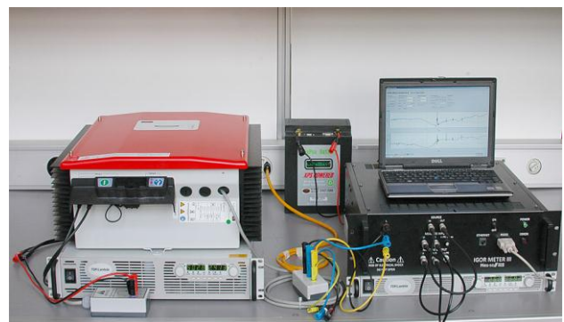
Fig. 1. Wideband grid impedance measurement set-up
