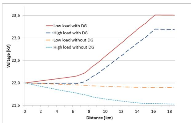
Figure 1 Example of voltage profile for a 22 kV line with a DG unit connected
