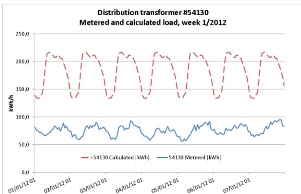
**Figure 5** Example of calculated and metered load profiles for a distribution transformer over a week (43 customers)
