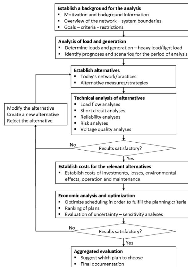
Figure 2 Planning methodology for electrical networks [5]
