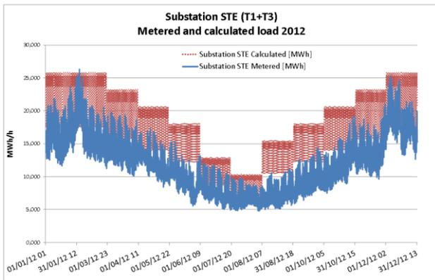
**Figure 3** Example of calculated and metered load profiles for a feeding substation over a year (4500 customers)
