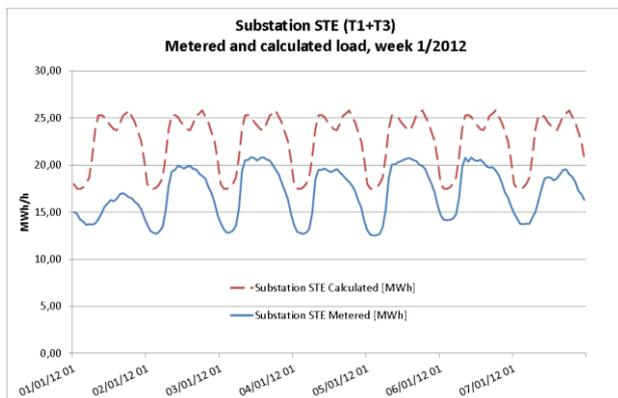
**Figure 4** Example of calculated and metered load profiles for a feeding substation over a week (4500 customers)
