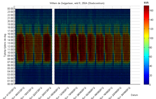
Figure 3: Power supplied to a city center feeder
