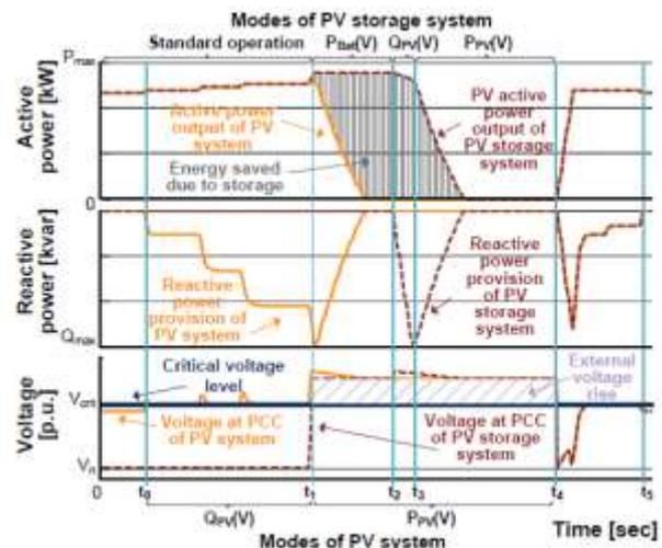
**Fig. 2.9: comparison of voltage control strategies for PV and PV storage systems (paper 1396).**
