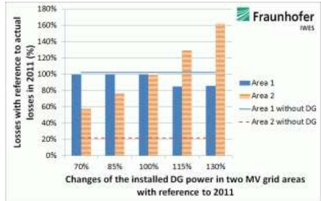
**Fig. 1.8: MV system losses variation with DG penetration (paper 1478).**
