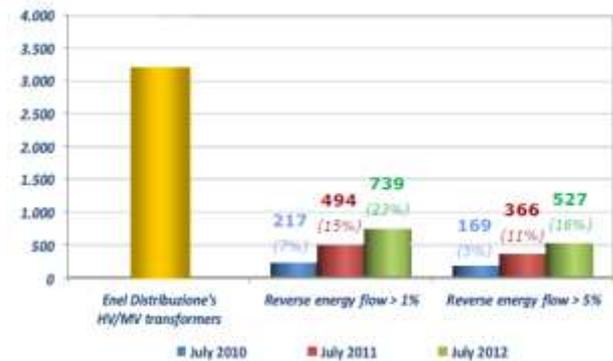
**Fig. 1.1: Reverse power flow in HV/MV transformers in Italian distribution system.**
