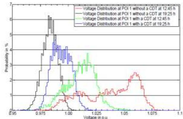
**Fig. 1.4: Impact of Controllable Distribution Transformer on voltage probability in LV network (paper 0575).**
