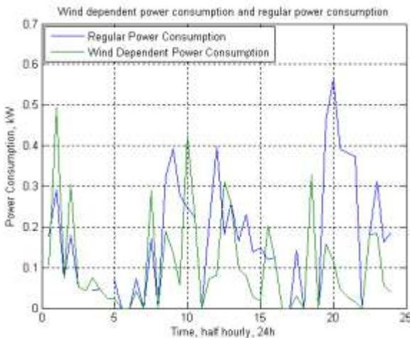
**Fig. 1.2: Impact on electrical demand for heating when optimised in accordance with wind power production (paper 0381).**
