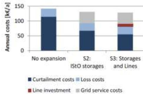
**Fig. 1.3: comparison of annual costs for no expansion, independent energy storage expansion and storage/line expansion plans (paper 0713).**
