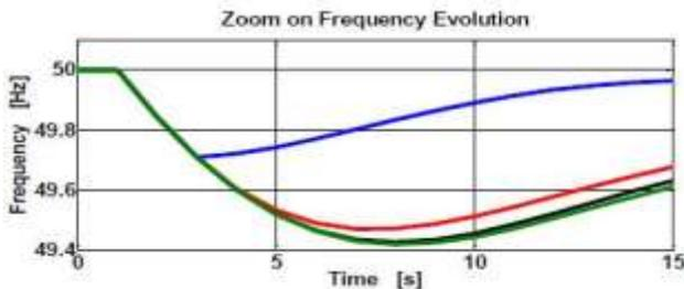
Fig. 3-4: Frequency evolution after a system disturbance (paper 0435).
