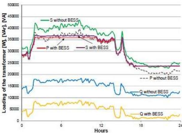
**Fig. 4-5: Peak shaving through battery energy storage system (BESS) (paper 1172).**
