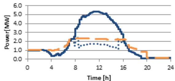
**Fig. 2.2: DG grid infeed before curtailment (solid line) and optimised VPP management of DG (dashed line) in comparison to standard curtailment measures (dotted line) (paper 0785).**
