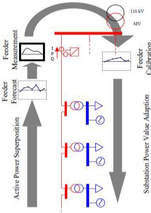
Fig. 2.4: RiesLing - Power flow forecast and calibration process (paper 0316).
