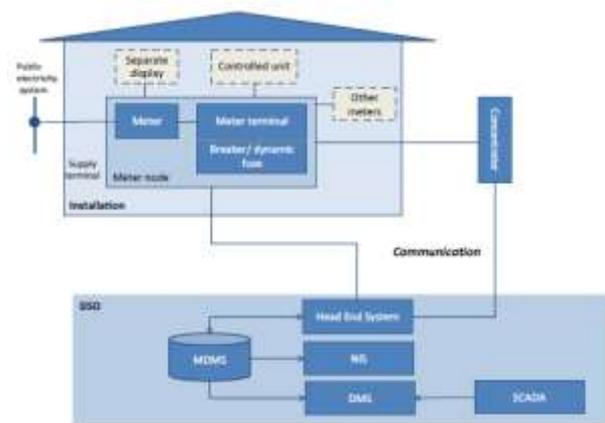
**Fig. 2.1: Smart Meter and ICT infrastructure in Norwegian trials (paper 1389).**
