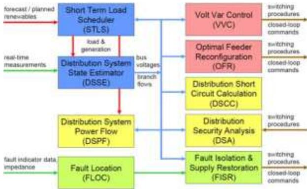
**Fig. 2.10: Distribution Network analysis applications (paper 0652).**
