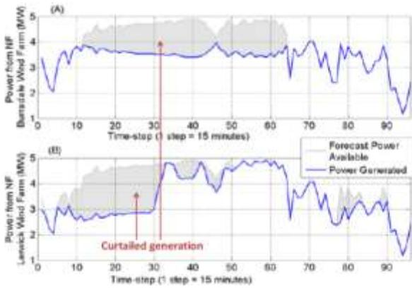
**Fig. 1.15: Generation curtailment for two generation locations in case study network after optimal scheduling of energy storage (paper 1327).**
