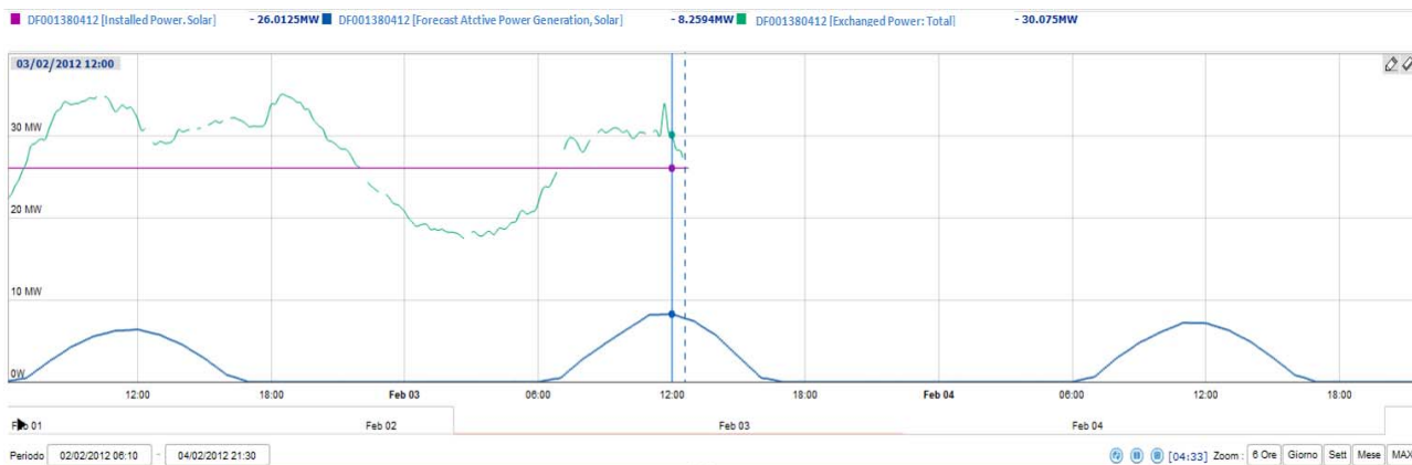
Fig. 2 - MAGO: forecasting of active power generation (bottom blue line) compared to other measures (web-based interface)
