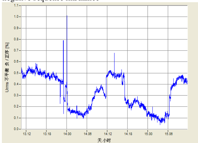
Figure * Negative sequence unbalanced three-phase curve
